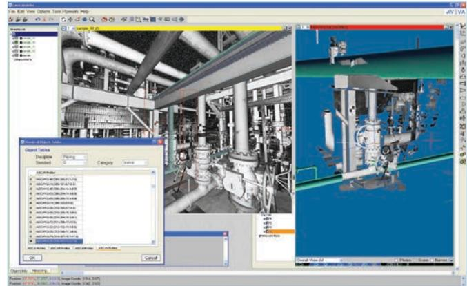
Laser Modeller produces the intelligent 3D as-built model by selecting a standard component from the PDMS catalogue, corresponding to the geometry derived from the laser scan data. In this example, we show pipework...
