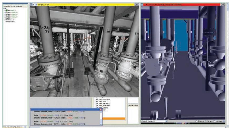
Photo-realistic laser scan data is a useful visualisation tool, but Laser Modeller adds huge engineering value, by enabling it to be converted directly into an intelligent, as-built, 3D PDMS plant model
